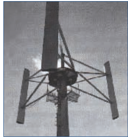
Figure 2: Left: The Globuan Darrieus turbine (a normal Darrieus). Right: a H-Darrieus turbine
